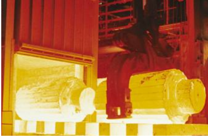
Metallurgical industry: forging furnace
